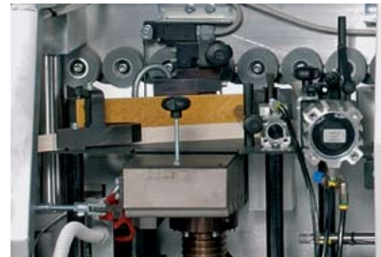
Teflon coated glue station with automatic temperature stand-by and 4.4 lb (2Kg) capacity.
