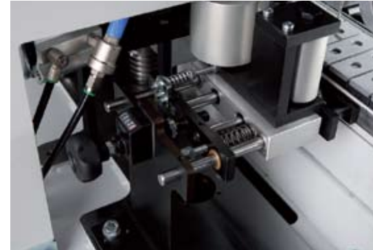
Pressure rollers with independent pressure adjustment and numerical indicators.
