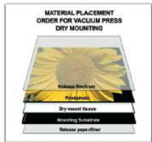
Illustration 11A: Top to bottom Material placement order in press
